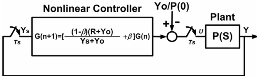
Fig.2 A Nonlinear Digital Controller.
