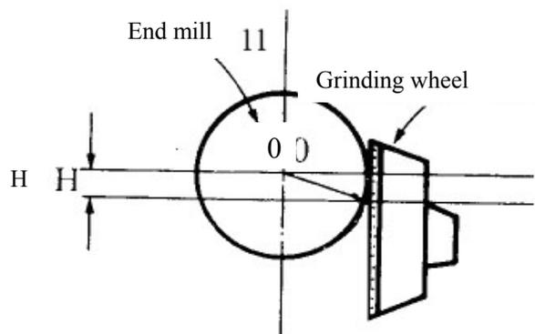
Fig.6 Height difference between the center of the endmill and that of the grinding wheel in grinding of flat relief angle
