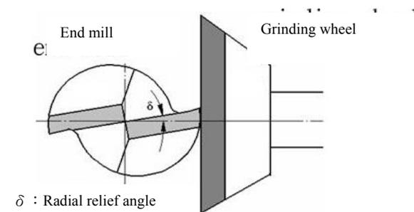
Fig.10 Schematic diagram for grinding of flat relief angle
