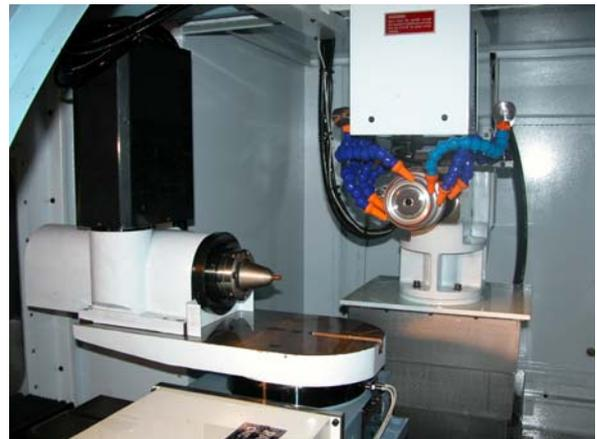
Fig. 9 Five-axis CNC tool grinder
