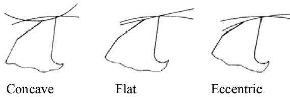
Fig.3 Common types of relief angle
