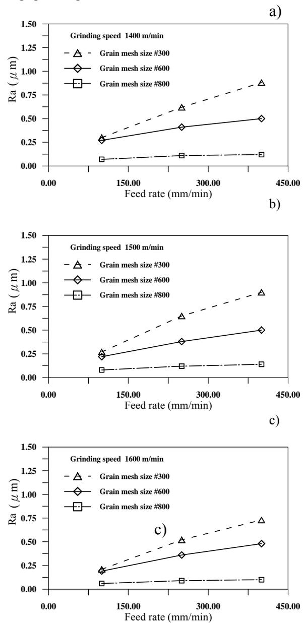
Fig.13 Effects of feed rate on surface roughness
