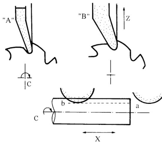
Fig.2 Grinding of radial rake angle
