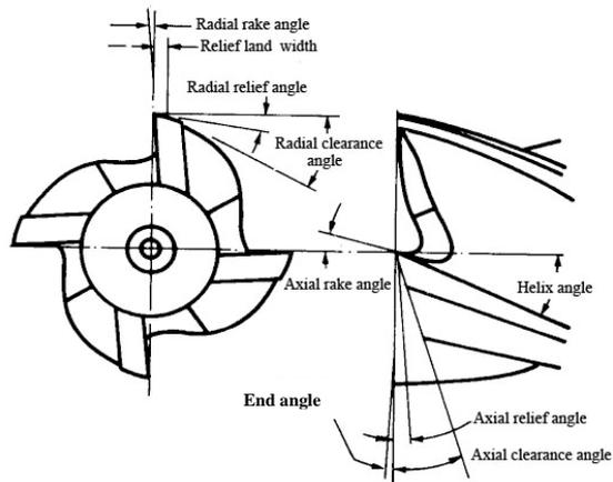
Fig.1 Various angles specified for endmills
