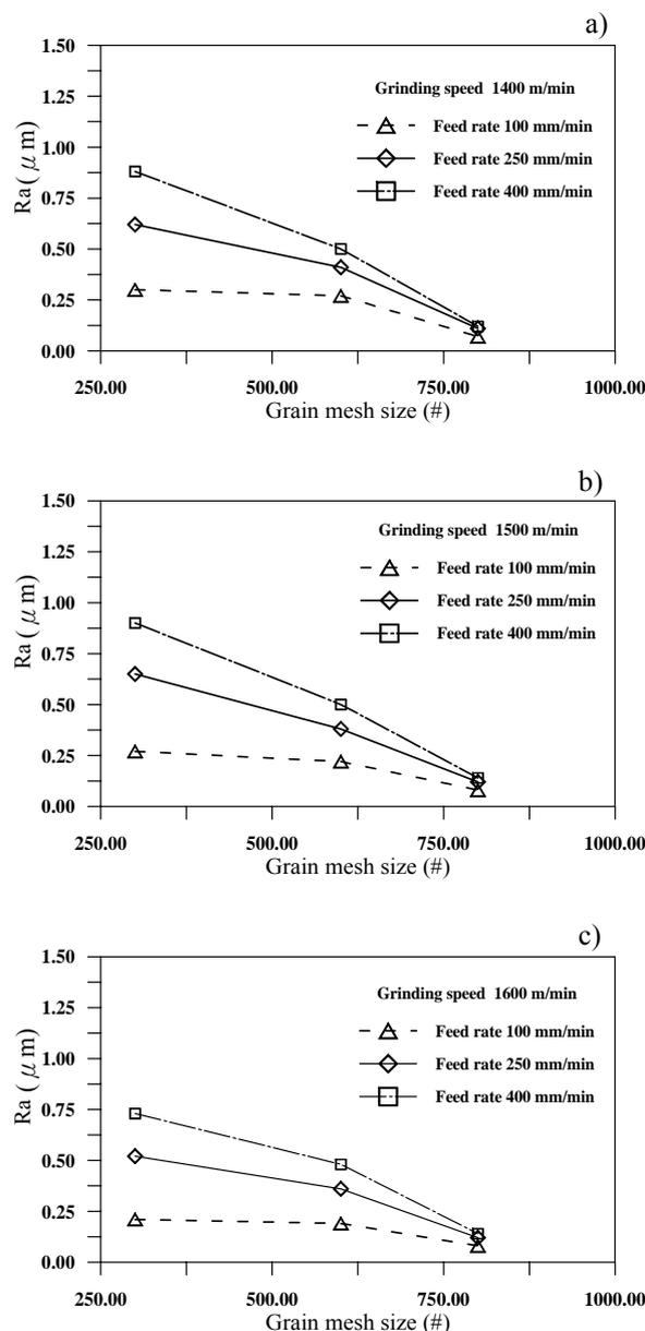
Fig.11 Effects of grain mesh size on surface roughness
