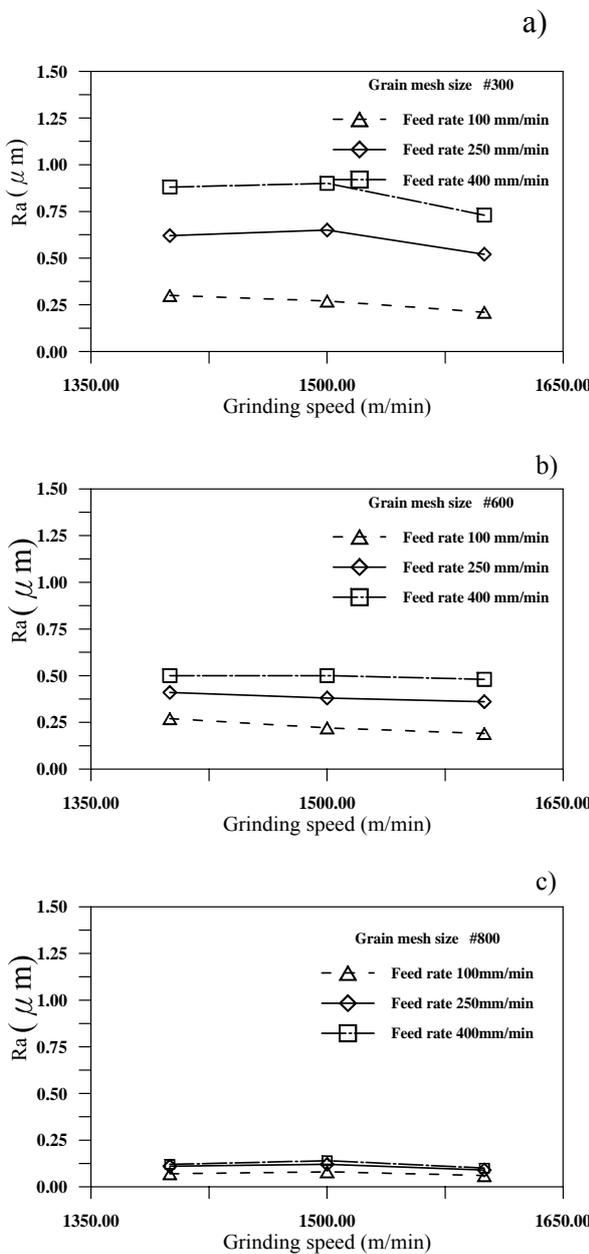
Fig.12 Effects of grinding speed on surface roughness
