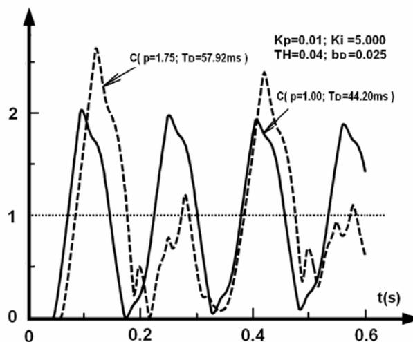
Fig.10 Maximal Pure Time Delay Simulation for p=1.0 and 1.75
