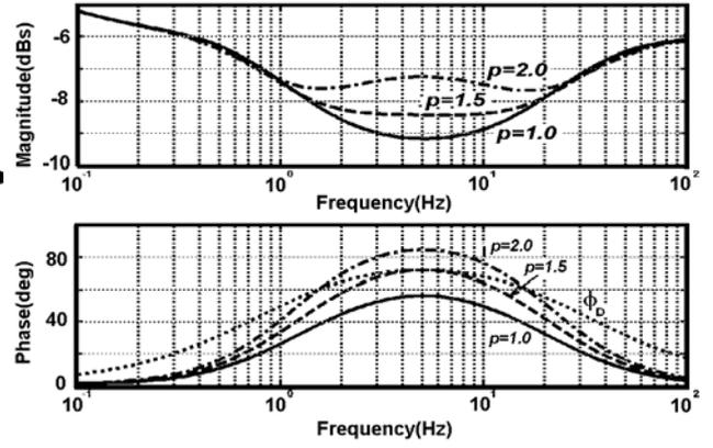
Fig.4 Frequency Responses of the VSSC Controller
