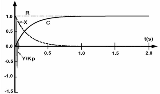
Fig.5 Time Responses of Example 1 with Bang-Bang Smoothing
