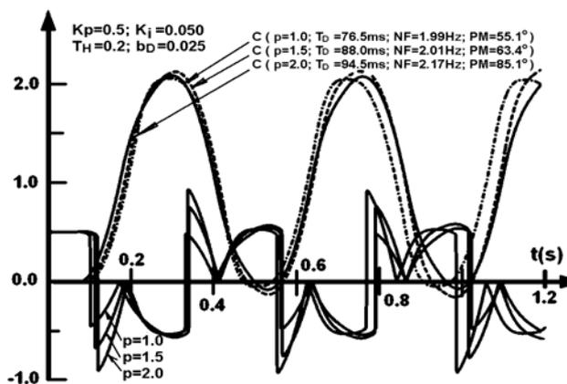
Fig.7 Maximal Pure Time Delay Simulation for p=1, 1.5 and 2.0
