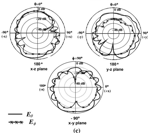
**Figure 3** Measured radiation patterns for the proposed antenna without and with two different curvatures at the appropriate resonant frequencies. (a) without curvature at  $f=5.73$  GHz, (b)  $\phi=95.5^\circ$ ,  $r=9$  mm at  $f=5.77$  GHz, (c)  $\phi=143.2^\circ$ ,  $r=6$  mm, at  $f=5.79$  GHz
