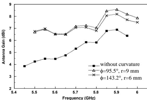
**Figure 4** Measured antenna gains for proposed antenna without and with two different curvatures
