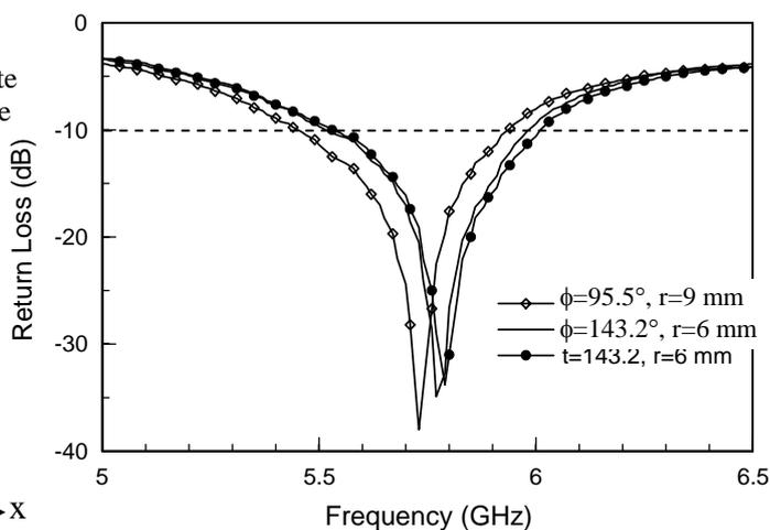
**Figure 2** Measured frequency responses of input return loss for proposed antenna without and with two different curvatures
