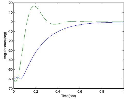
Fig.4 (a) Position error of link 1
